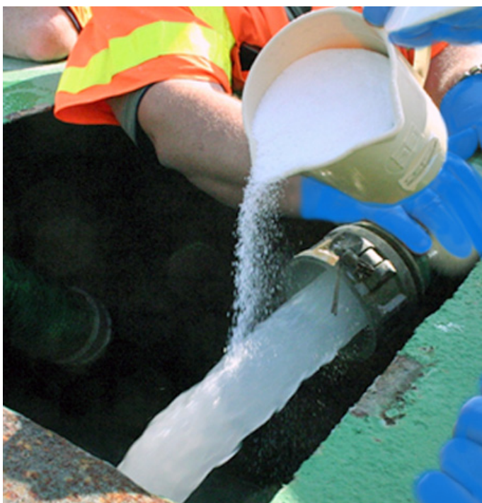
FIGURE 26 GRAVITY FEEDING POLYMER INTO A STREAM OF RECIRCULATED POLYMER FLUID
