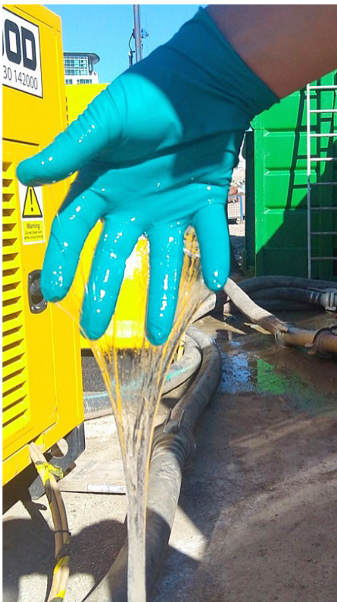
FIGURE 3.B SYNTHETIC POLYMERS USED IN SUPPORT FLUIDS
