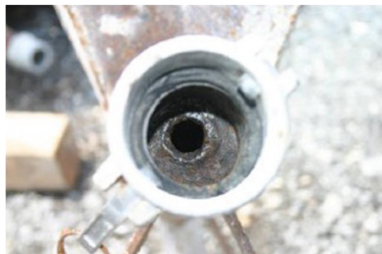
FIGURE 27 A SIMPLE VENTURI HOPPER ASSEMBLY: 50MM [2 IN] SUPPLY LINE REDUCED TO 19MM [3/4 IN] TO FORM NOZZLE (TOP); HOPPER WITH NOZZLE PORT AT THE BASE (MIDDLE); AND SCHEMATIC OF SIMPLE VENTURI HOPPER MIXING SYSTEM (BOTTOM)
