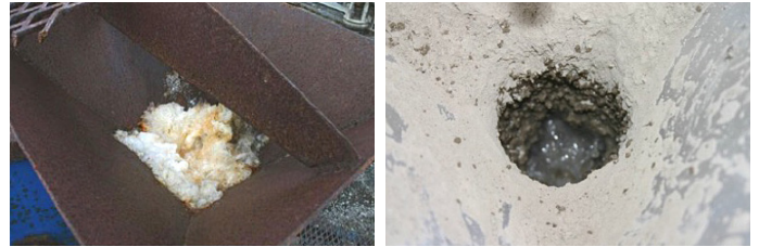
FIGURE 29 HOPPER CLOGGED WITH WETTED POLYMER (LEFT); BUILD-UP OF PARTIALLY WETTED MINERAL PRODUCT (RIGHT)
