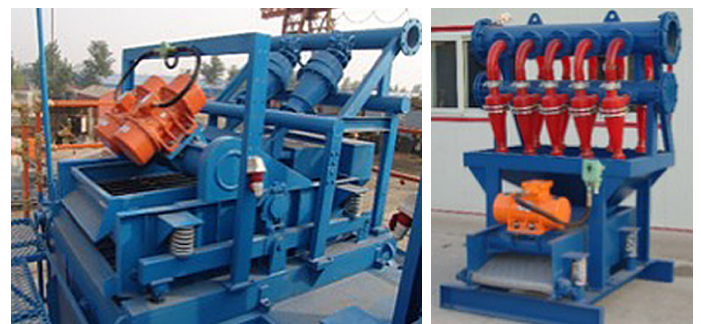
FIGURE 35 EXAMPLES OF DESANDER CYCLONES (TOP LEFT), DESILTER CYCLONES (TOP RIGHT) AND CENTRIFUGE (BOTTOM).
