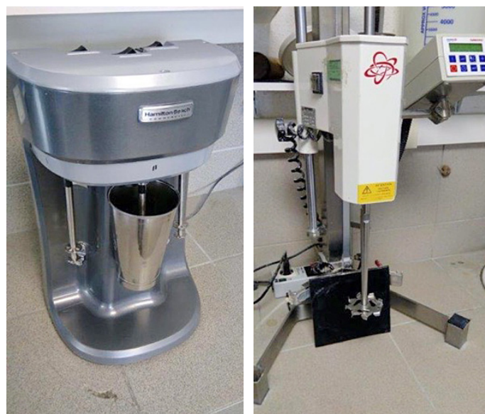
FIGURE 20 HAMILTON BEACH MIXER (LEFT) AND RAYNERI MIXER (RIGHT), FOR LABORATORY USE ONLY
